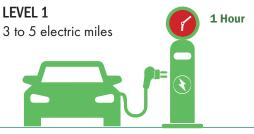
Requires access to a 120-volt outlet in an area where you can recharge the car overnight (or have a qualified electrician install one in a convenient location).
