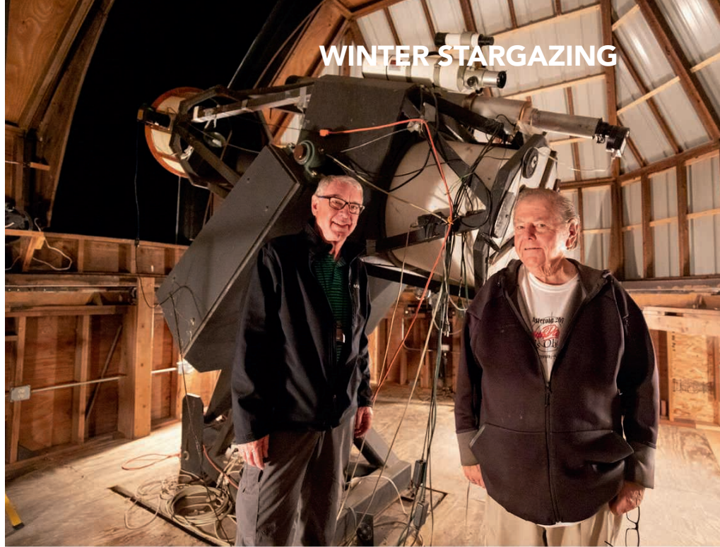
Photographer Bob Rossiter and Ron Dyvig are shown with the 26-inch Newtonian Reflector telescope at Badlands Observatory.
